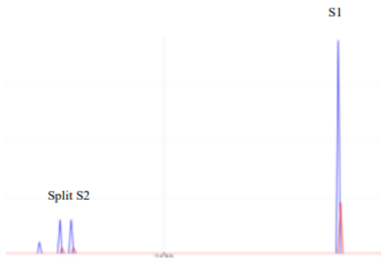
Fig 6. Sound signal of split S2 obtained from microcontroller
