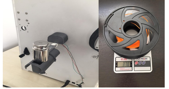
Figure 3: Measurement of filament weight with precision scale and calibration of the system performed with standard weights
