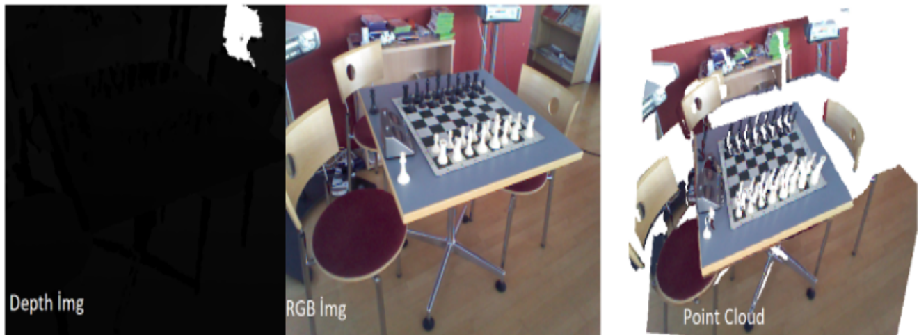
Figure 2: RGB-D image to point cloud
