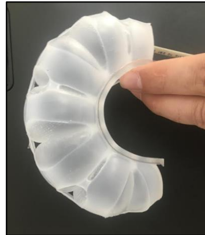
Figure 7. Actuation and Grasping Geometry of the Soft Finger
