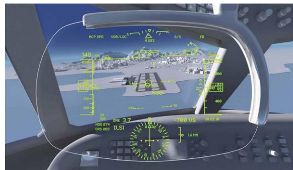
Figure 3 - Head-up Displays (HUDs) in aviation (adapted from https://www.flyingmag.com/how-it-works-head-up-display/ retrieved on November 20, 2020)
