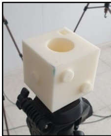
Figure 5. Model of Rigid Body Mockup within Motion Capture Workspace
