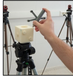
Figure 6. Measurement Procedure via Calibrated Stylus
