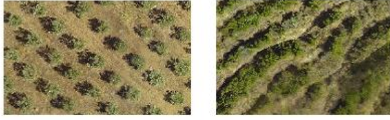
Figure 1. Comparison of an area with multiple (left) and insufficient overlapping images (right)
