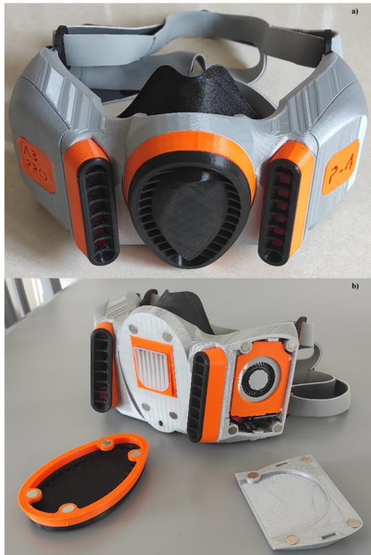
Figure 4: a) Completed assembly of the mask. b) Removable covers of the mask using the magnetic assembly method.
