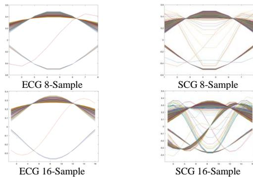
**Figure I.** Sample PSV Sets for ECG & SCG Signals w/8- and 16-Sample Frame Lengths
